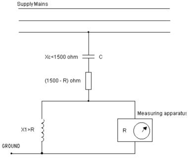
Circuit for RF voltage measurement on supply mains (subclause 12.2)
