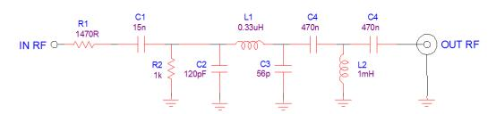
Fig. 2-3 PMM SHC-2/1000 passive probe schematics
